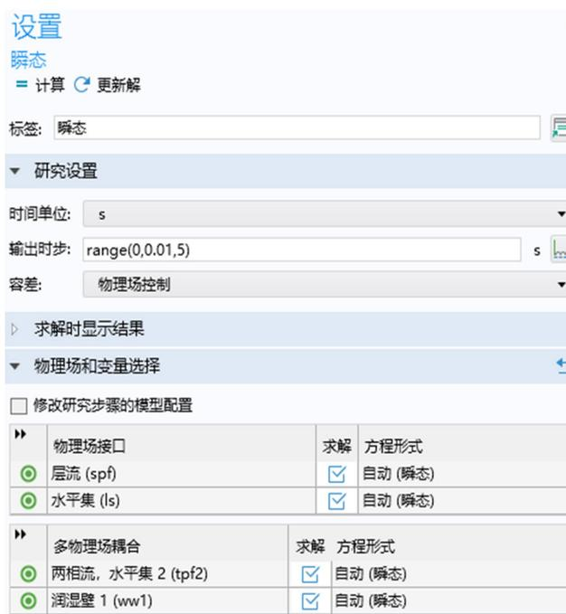
Figure 10. Transient solver timestep settings
