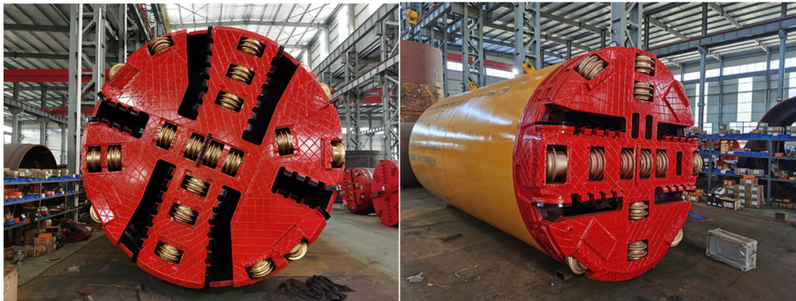
Figure 2. Selection diagram of domestic slurry balance pipe jacking machine (Complete Machine) 图 2. 国产泥水平衡顶管机整机选型图
