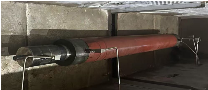
Figure 20. Hydraulic and electronic control joint commissioning test fixture 图 20. 液控与电控联调测试工装
