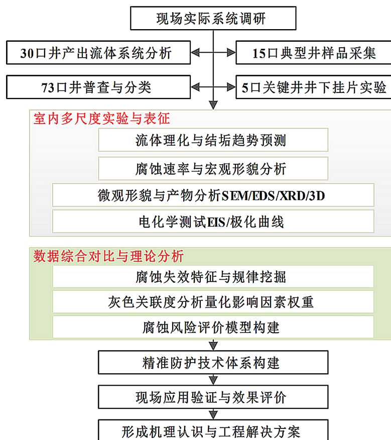
Figure 1. Multi-scale integrated research framework (field investigation → laboratory experiments → theoretical analysis) 图 1. 多尺度综合研究方法体系(现场→实验→理论分析)
