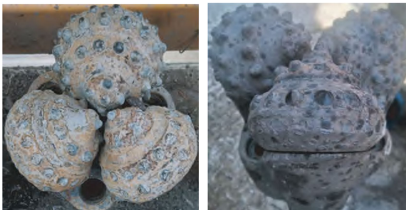
Figure 1. Photo of severely worn bit encountering high hardness and strong abrasiveness formation 图 1. 钻头钻遇硬度高、研磨性强严重磨损照片
