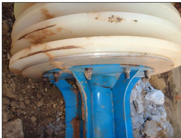
Figure 7. Two-gauging disc pig with additional steel gauging disc 图 7. 加装钢质测径板后的双测径板清管器
