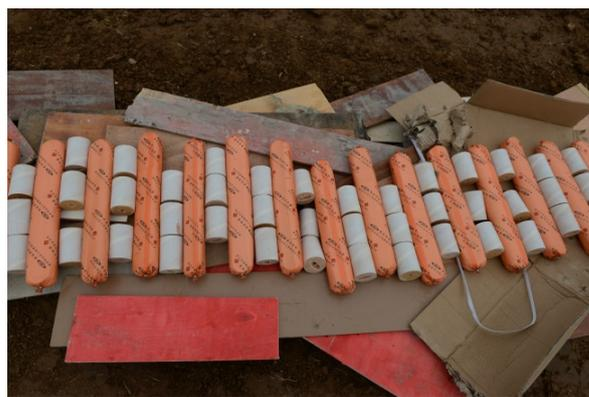
Figure 3. Various explosives mix and match layout drawing
