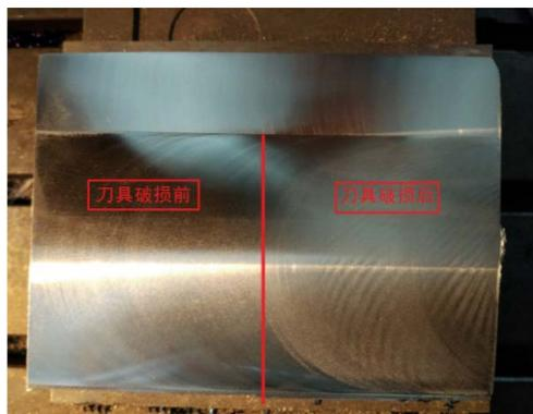
Figure 4. The surface appearance of the workpiece where the tool damage occurred
