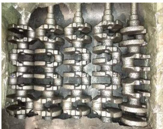
**Figure 13.** Crankshaft blank
