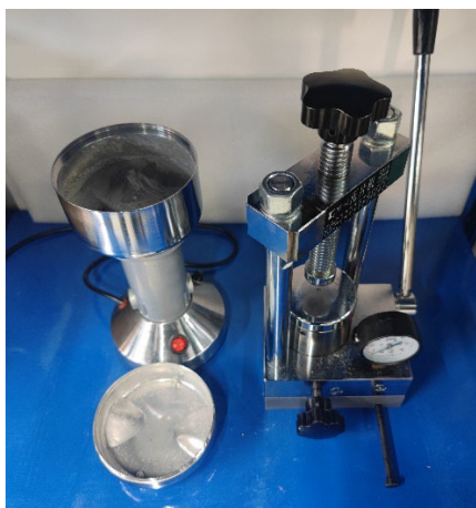
Figure 4. Equipment for stone powder pulverization and tablet compression
