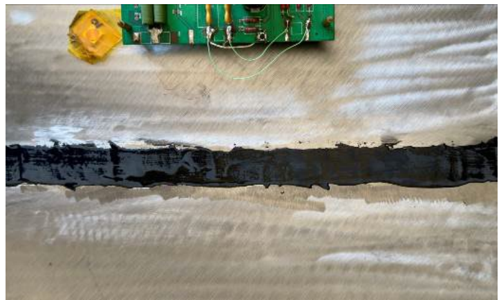
Figure 14. Photograph of the weld coated with the magnetostrictive layer 图 14. 涂有磁致伸缩涂层的焊缝实物图
