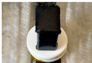
Figure 15. Photograph of the weld coated with the magnetostrictive layer
