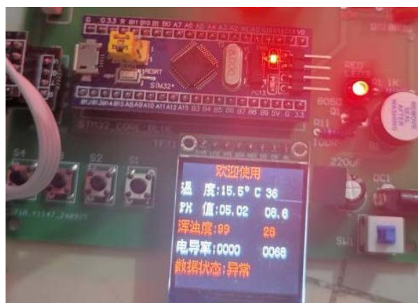
Figure 12. Warning function test diagram
