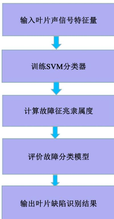
**Figure 2.** Implementation steps of wind turbine blade defect identification model based on SVM
