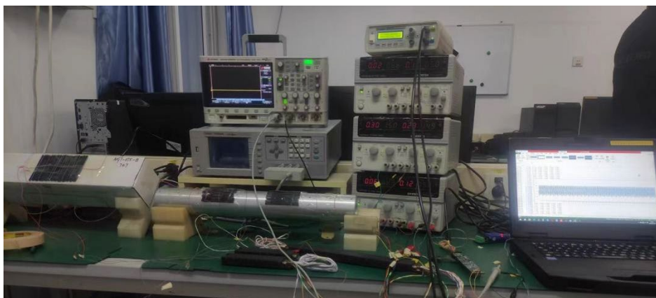
Figure 13. Diagram of the azimuthal electromagnetic wave resistivity principle system test 图 13. 方位电磁波电阻率原理系统测试图
