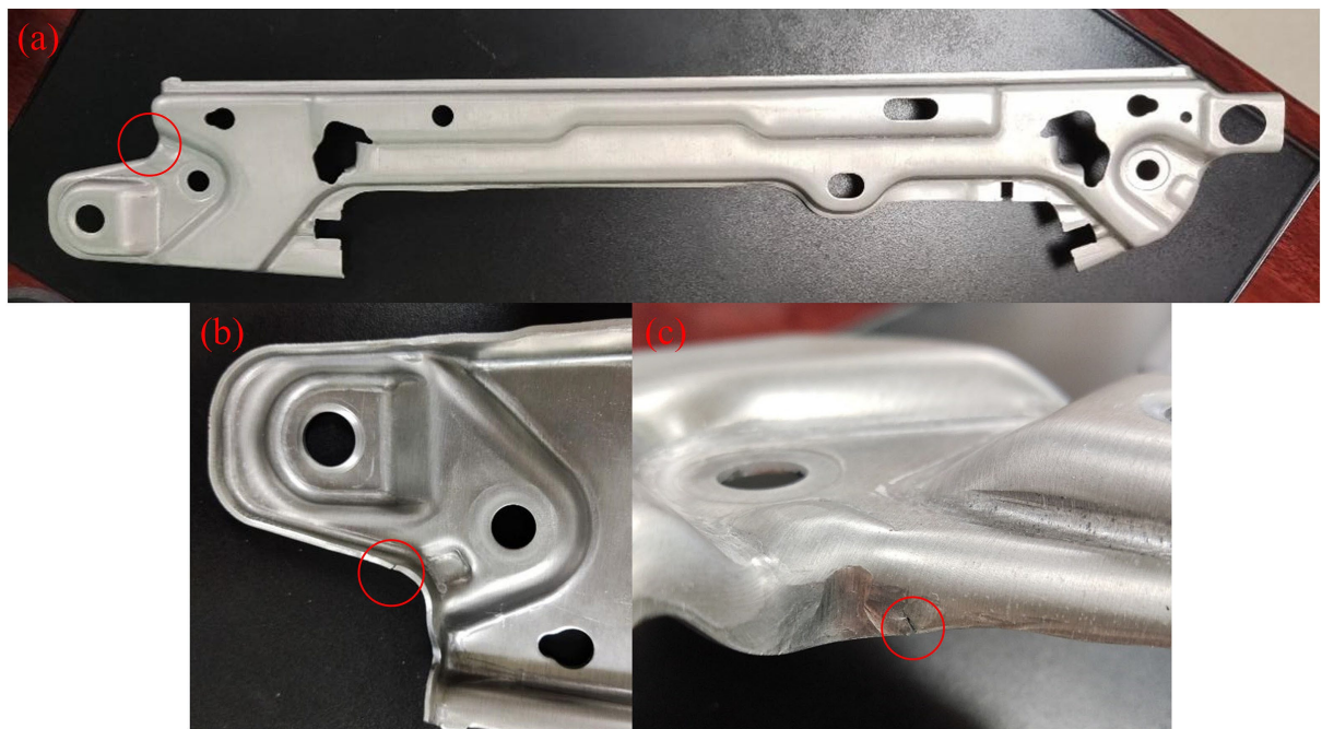
Figure 1. Defect locations of the part: (a) Overall morphology; (b) Local morphology of the back side; (c) Local morphology of the side face
