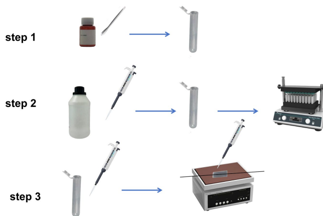
Figure 2. Fabrication process of ZIF-8 coating via drop-coating
