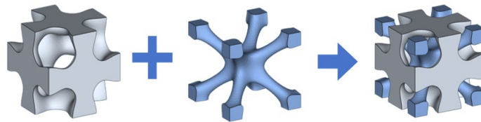
Figure 1. Design diagram based on TPMS interpenetrating lattice structure 图 1. 基于 TPMS 互穿晶格结构设计图
