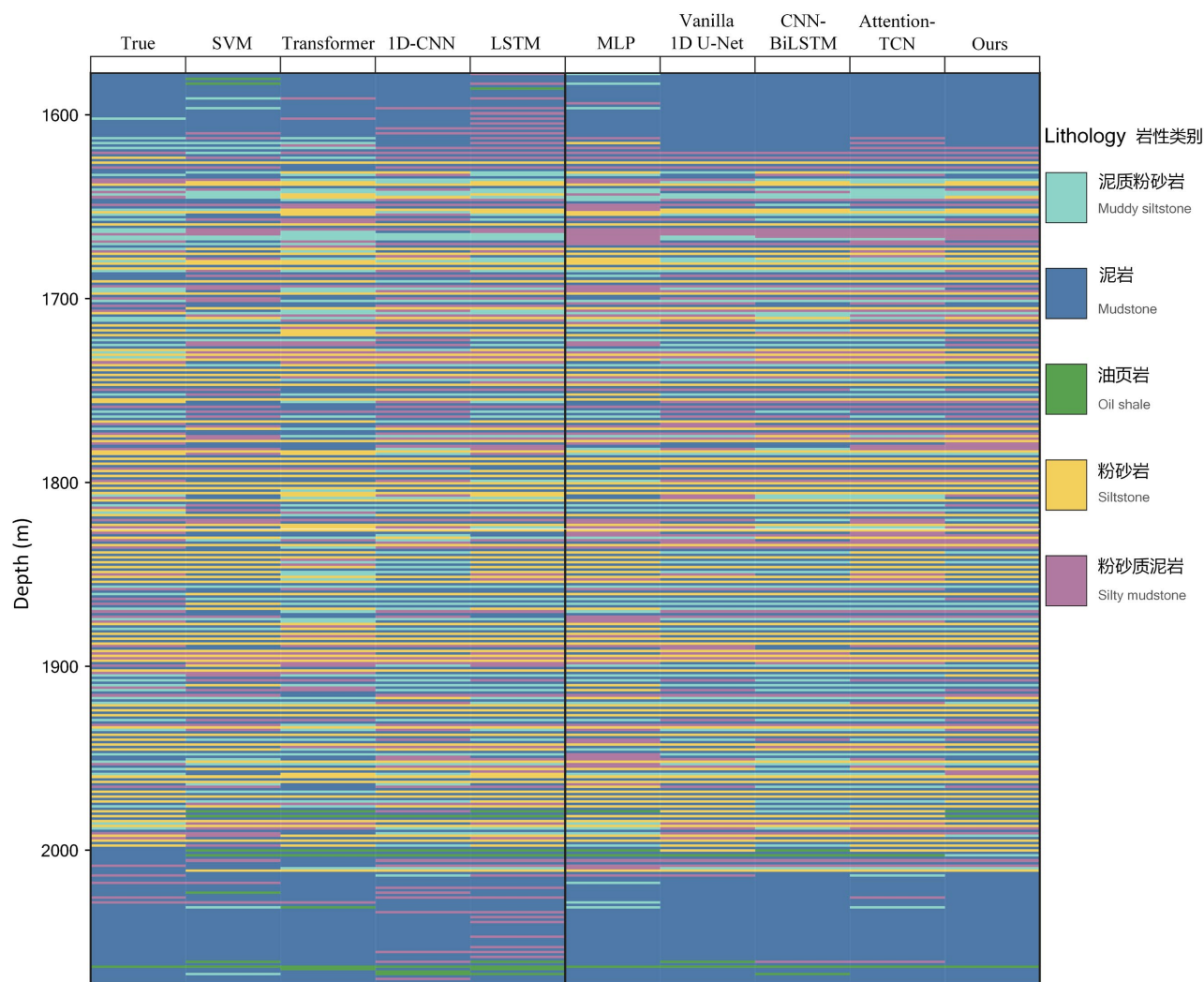
Figure 9. Comparison of true lithology and lithology predictions of different models along depth in well J393
