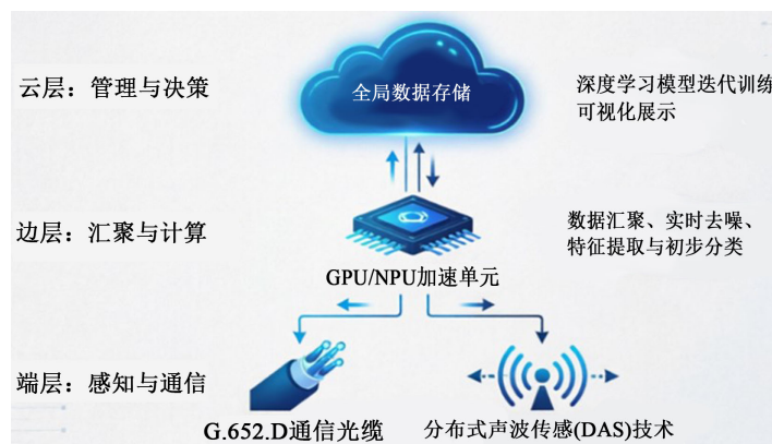
Figure 1. Collaborative architecture diagram of “Terminal-Edge-Cloud” with integrated sensing and communication 图 1. 通感一体化的“端 - 边 - 云”协同架构图
