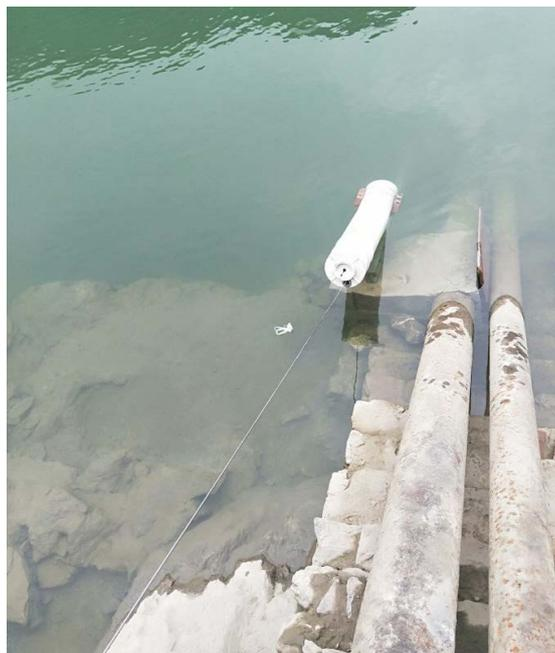
Figure 5. The field installation diagram of eccentric buoy
