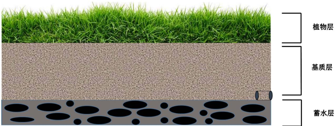
Figure 2. Typical structure of green roof
