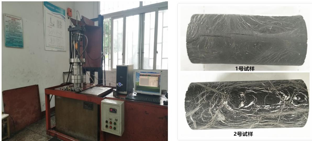
**Figure 2.** Three axis percolation test machine and experimental sample
