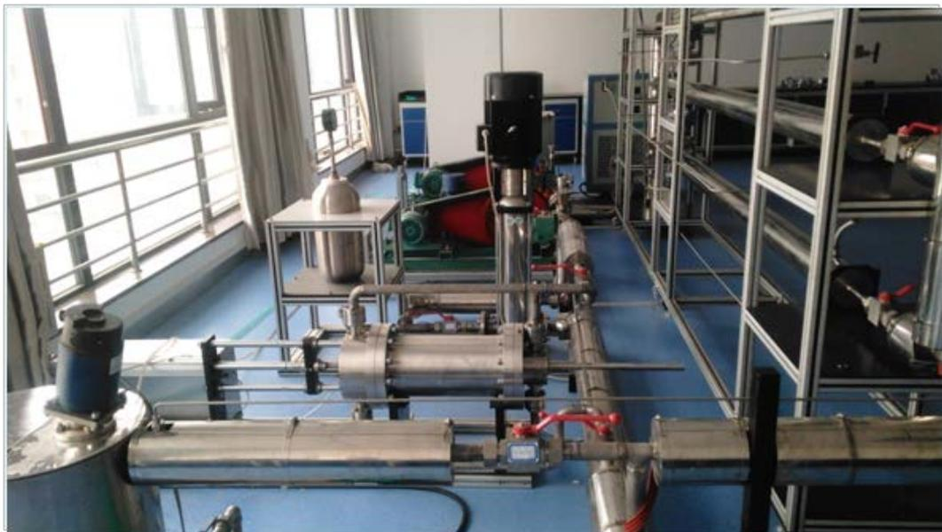
Figure 2. Flowing friction testing equipment
