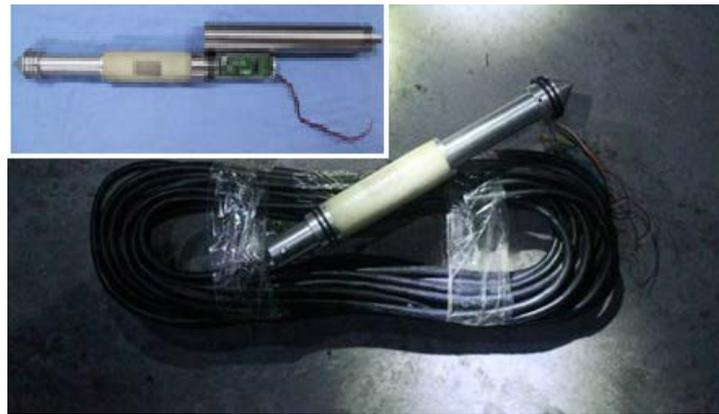
**Figure 2.** Hollow inclusion stress meter
