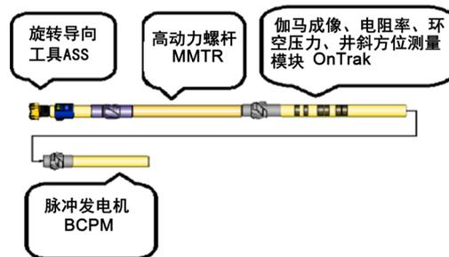
**Figure 2.** Rotate the geosteering tool
