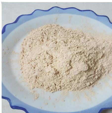
**Figure 4.** Ding 44108A-2 sandstone rock powder for acid rock dissolution experiment
