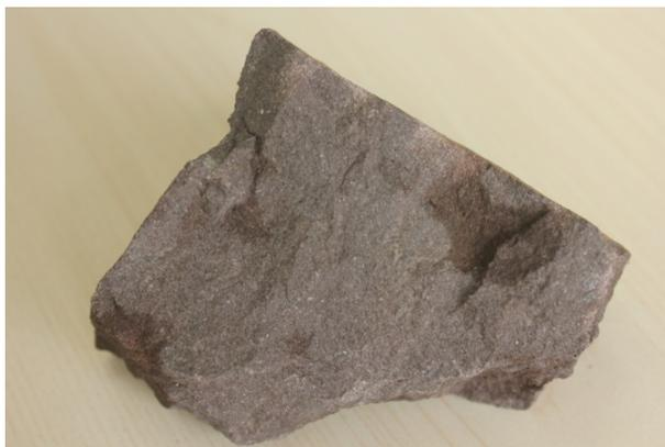
**Figure 3.** Ding 44108A-2 sandstone for acid rock dissolution experiment
