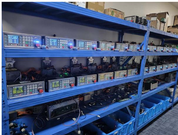
**Figure 5.** The actual scene diagram of the hardware self-check experimental platform for the hydraulic support controller
