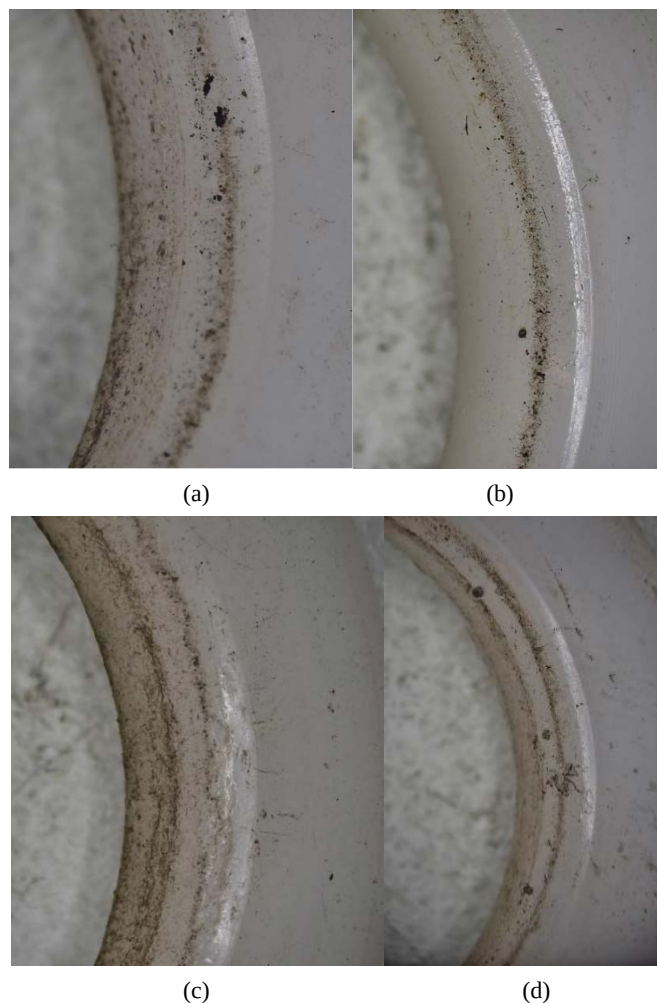
Figure 3. Enlarged picture of sealing surface of valve seat (a) sealing surface of No.1; (b) sealing surface of No.3; (c) sealing surface of No.4; (d) sealing surface of No.5
