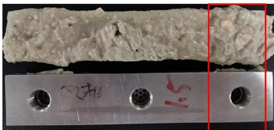
Figure 9. Fracture module plugging effect diagram
