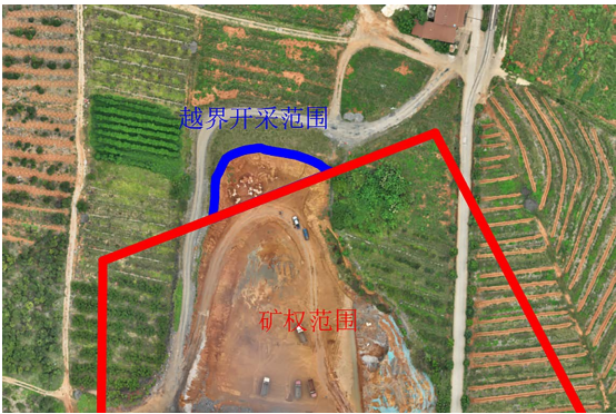
Figure 6. Confirming the part of cross-border mining 图 6. 确认越界开采部分
