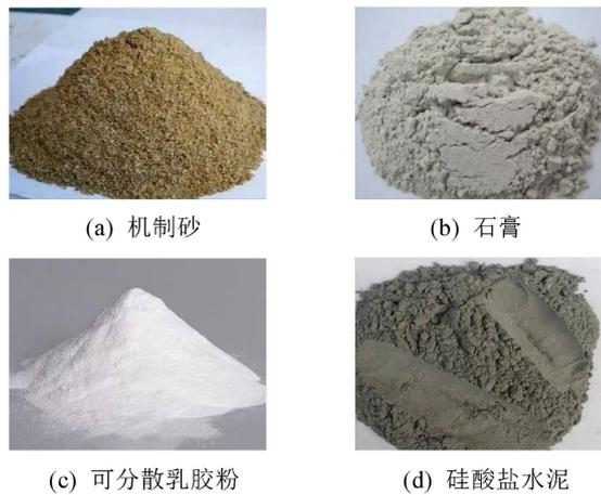
**Figure 1.** Materials for physical model test
