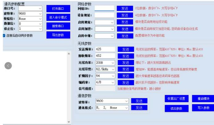
Figure 4. Configuration diagram of LoRa wireless transmission module
