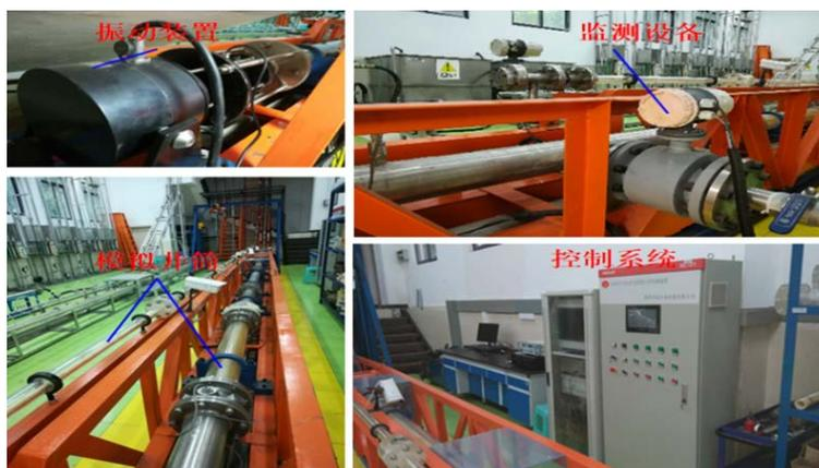
Figure 3. Indoor simulation test platform
