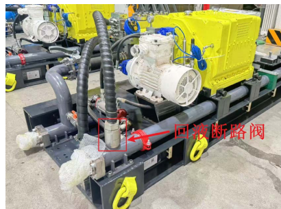
Figure 2. Photograph of the check valve in the pump station 图 2. 回液断路阀在泵站的实物图
