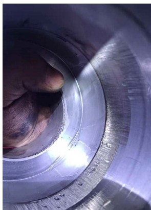
Figure 9. Diagram of sticking on the valve seat guide surface 图 9. 阀座导向面卡涩图
