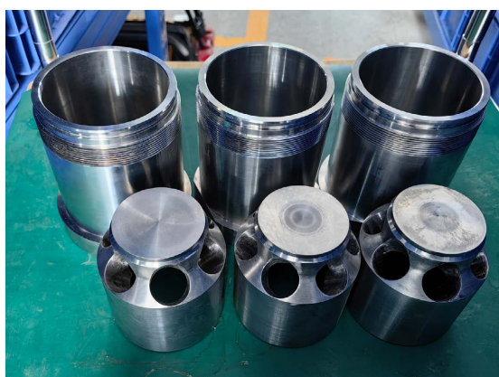
Figure 13. Prototype of two-stage throttling check valve 图 13. 二级节流回液断路阀样机
