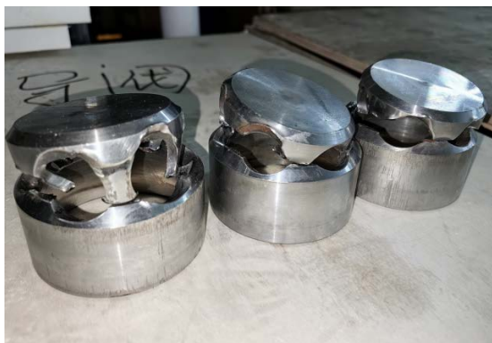
Figure 10. Photograph of the fractured valve spool 图 10. 阀芯断裂图
