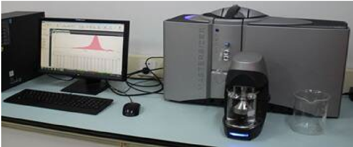
Figure 1. Mastersizer 3000 laser diffraction particle size analyzer 图 1. Mastersizer 3000 激光衍射粒度分析仪
