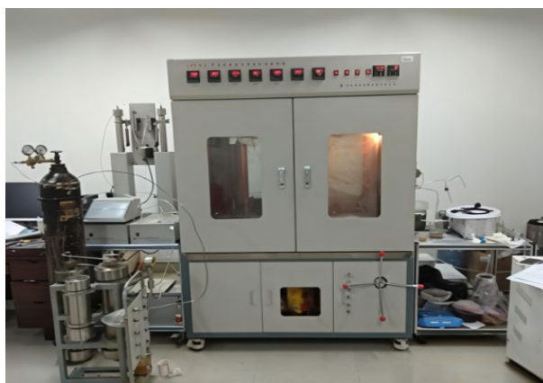
Figure 2. LDY-II multifunctional displacement physical simulation system 图 2. LDY-II 型多功能驱替物理模拟系统
