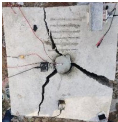
Figure 6. Reservoir fracture morphology after fracturing [20]
