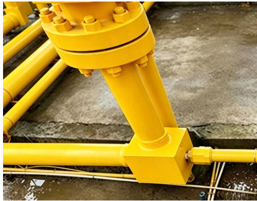
Figure 6. Installation position of atomization defoaming intelligent filling device 图 6. 雾化消泡智能加注装置安装位置
