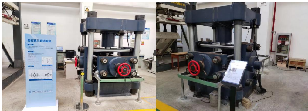
Figure 1. Microcomputer controlled triaxial fully automatic detection and testing platform 图 1. 微机控制三轴全自动检测试验平台
