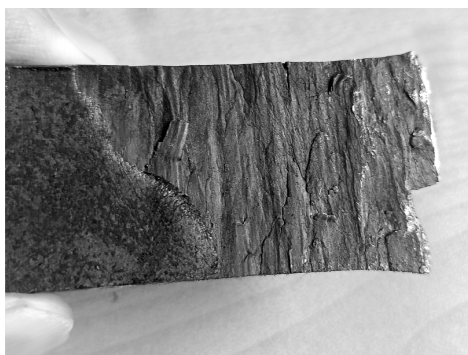
Figure 2. Near surface morphology of tensile abnormal fracture sample
