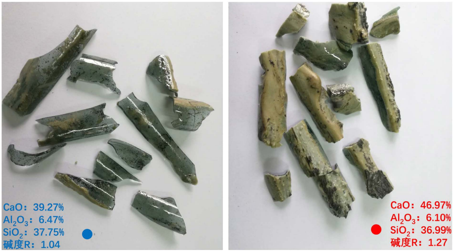
Figure 2. Color of final slag state before and after adjustment 图 2. 调整前后精炼终渣状态颜色
