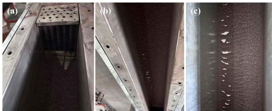
Figure 8. Ash distribution on the bottom surface of the downstream channel of the heat exchanger specimen: (a) near the outlet of the specimen; (b) downstream of the specimen; (c) localized distribution downstream of the specimen
