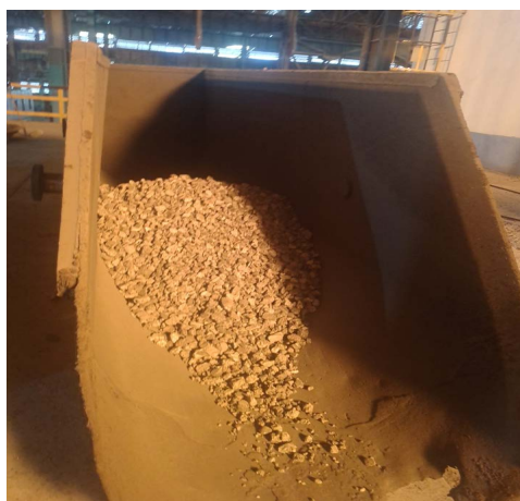
Figure 3. The material is baked on the AOD stove table 图 3. 原料在 AOD 炉台烘烤
