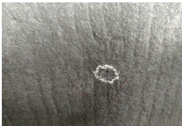
Figure 2. Defect of porosity in J5 stainless steel billet 图 2. J5 不锈钢钢坯气孔缺陷
