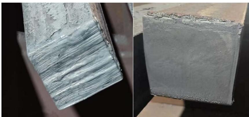
**Figure 6.** Comparison of cast strand cross-section before and after modification
