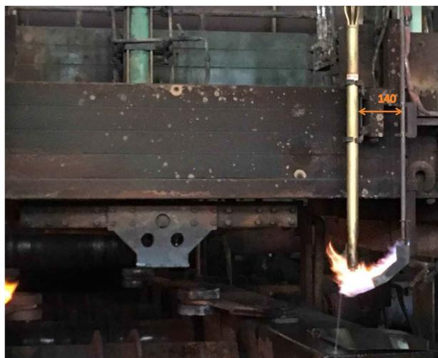
**Figure 2.** Schematic diagram of the original flame cutting machine and pilot flame distance
