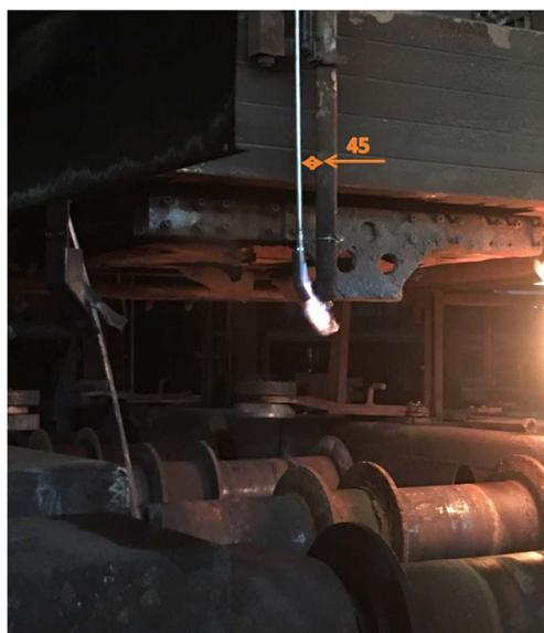
**Figure 3.** Post-modification flame cutting machine equipment diagram
