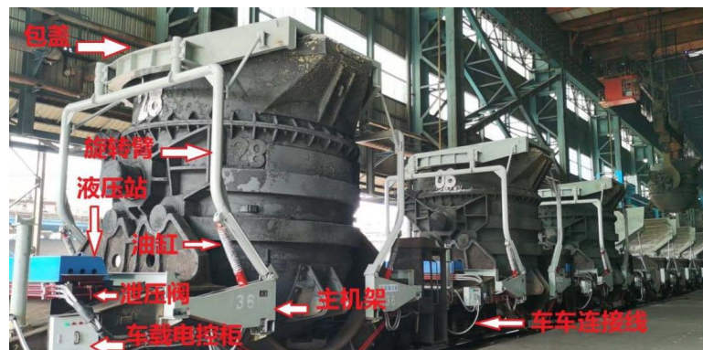
Figure 4. Hydraulic cantilever-type hot metal ladle cover system 图 4. 液压悬臂式铁水罐加盖系统
