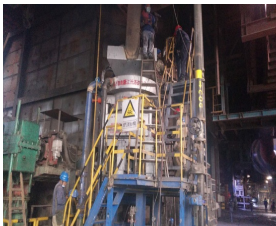
Figure 6. Alloy preheating operation diagram 图 6. 合金烘烤工作图
