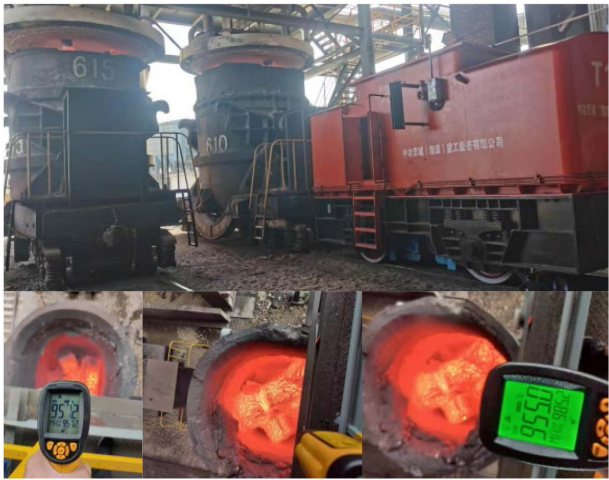
Figure 5. Hot metal ladle scrap preheating system
