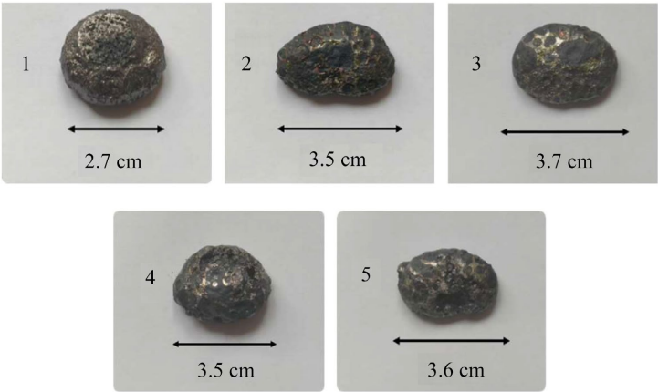
Figure 6. Effect of CaF 2 addition on the morphology 图 6. CaF 2 用量对还原铁形貌影响
