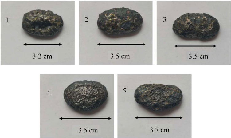
Figure 8. Effect of temperature on the morphology 图 8. 温度对还原铁形貌影响
