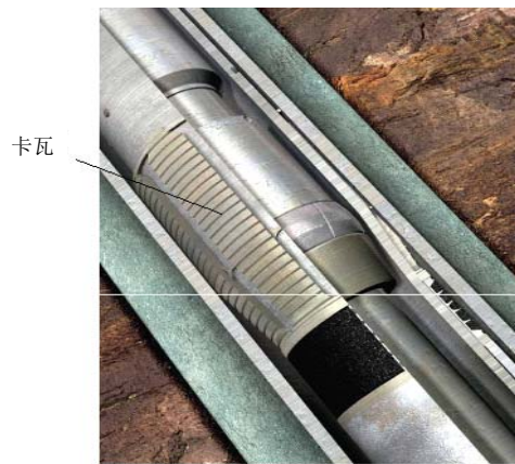
Figure 5. Structure of Baker Hughes's ELH 图 5. 贝克休斯膨胀尾管悬挂器示意图
