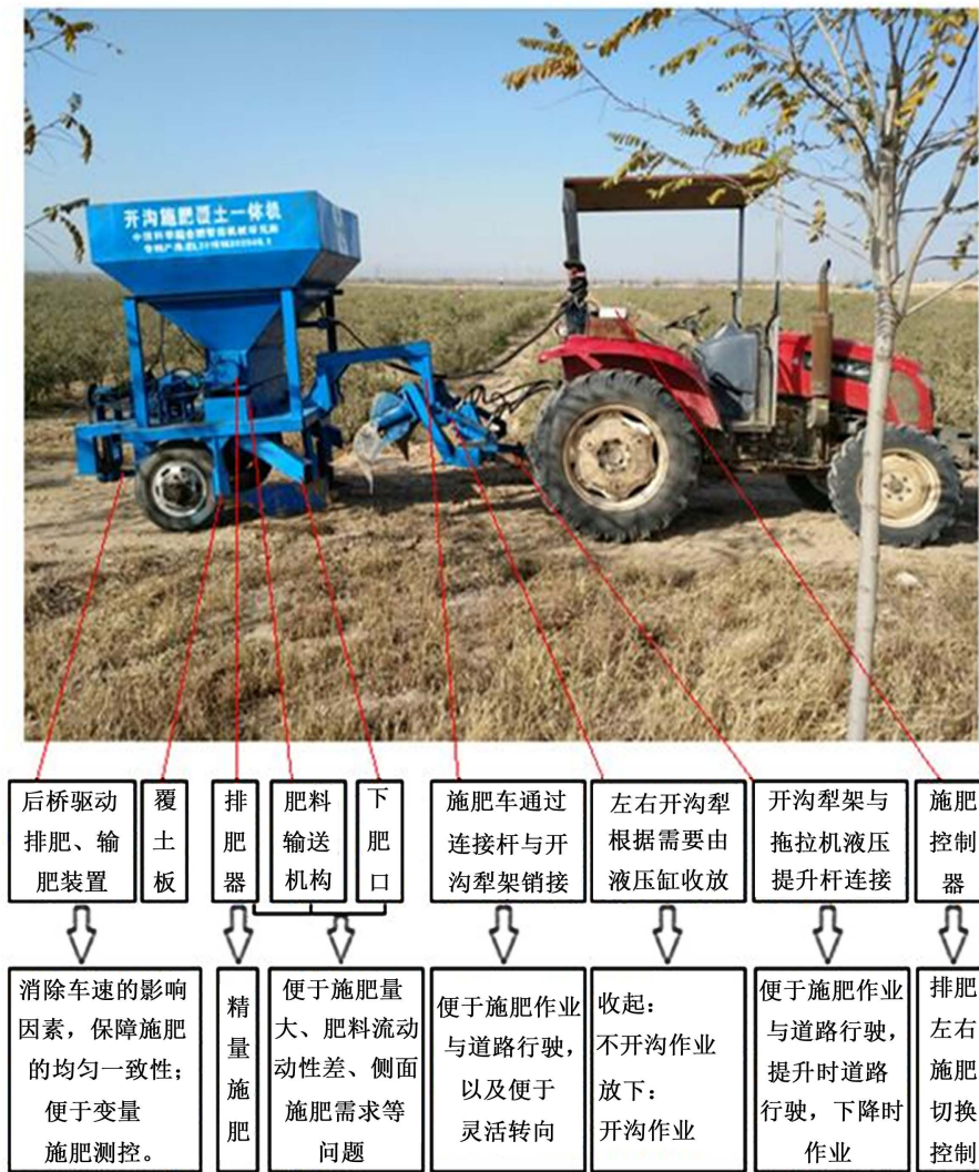
Figure 1. Overall structure illustration 图 1. 整体结构说明图
