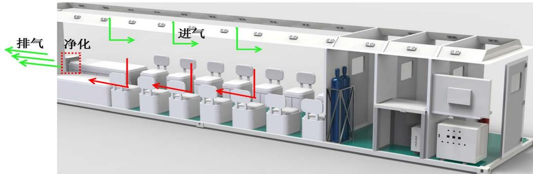
Figure 3. Air flow in the cabin
