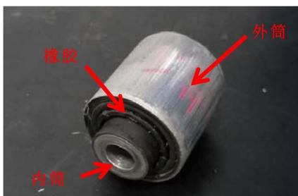
**Figure 2.** Structural drawing of cylindrical bushing
