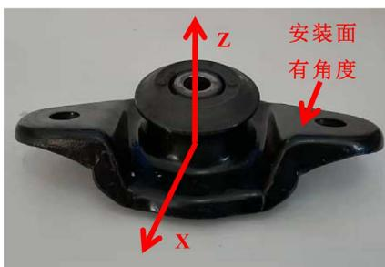
**Figure 3.** Shock absorber upper support bushing
