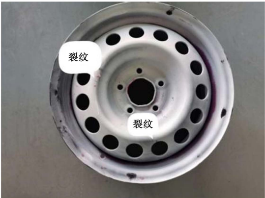
Figure 3. Cracks in ventilation holes after flaw detection 图 3. 探伤后通风孔裂纹
