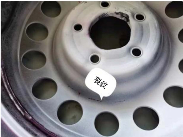
Figure 4. Cracks in the middle position of the ventilation hole and the bolt hole after flaw detection 图 4. 探伤后通风孔与螺栓孔中间位置裂纹
